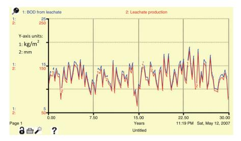
Fig. 12.10 Simulated leachate production (mm) and BOD  $(kg/m^2)$  from leachate for a time horizon of 30 years
