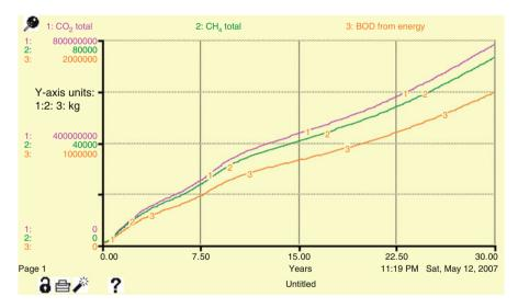
Fig. 12.9 Simulated CO<sub>2</sub> total, CH<sub>4</sub> total and BOD from energy for a time horizon of 30 years
