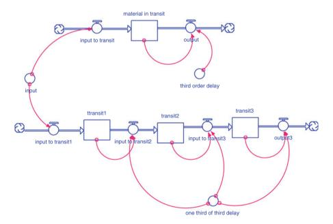
Fig. 4.14 Flow diagram of material delay
