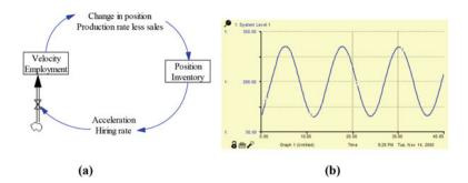
Fig. 1.11 (a) Causal loop diagram of a second order system and (b) dynamic behaviour of a second order feedback system
