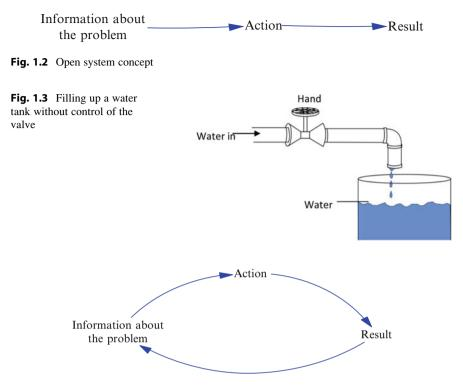
Fig. 1.4 Closed loop system concept
