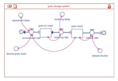
Fig. 4.18 Stock-flow diagram of grain storage system
