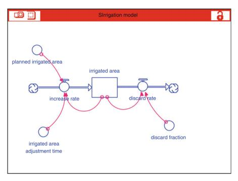
Fig. 2.6 Stock-flow diagram of the irrigation model
