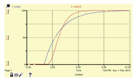
Fig. 4.15 STEP response of first-order material delay (output) and third-order material delay (output 3)
