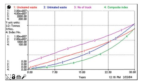
Fig. 12.11 Simulated uncleared waste, untreated waste, number of trucks and composite index with increase in collection capacity for a time horizon of 30 years
