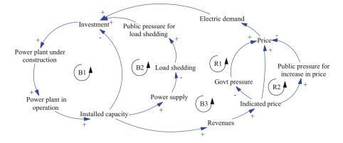
Fig. 3.11 Causal loop diagram of electricity supply system
