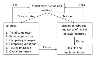
Fig. 6.7 Logical sequence of behaviour pattern tests
