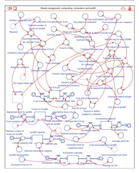
Fig. 12.2b STELLA flow diagram of solid waste management system dynamics—composting, incineration and landfill
