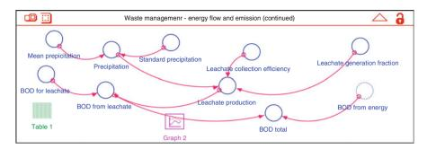
Fig. 12.2d STELLA flow diagram of solid waste management system dynamics—energy flow and emissions
