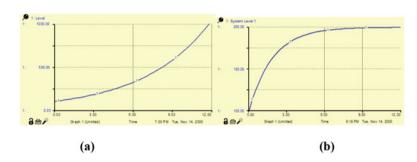
Fig. 1.9 Dynamic behaviour of (a) positive feedback and (b) negative feedback systems
