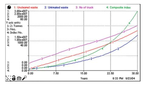
**Fig. 12.12** Simulated uncleared waste, untreated waste, number of trucks and composite index with increased collection capacity, treatment capacity and landfill capacity for a time horizon of 30 years
