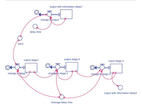
Fig. 4.12 Flow diagram of information delay
